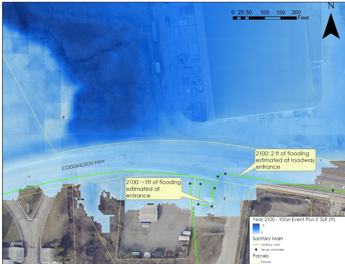
Figure 4. Projected water surface elevations around the Coddington Highway Pump Station for a 100-year coastal flooding event in the year 2100, factoring in 5 ft of sea level rise (SLR). Flood projections calculated by Coastal Resources Management Council (CRMC) STORMTOOLS, presented as water depth in feet above grade.
