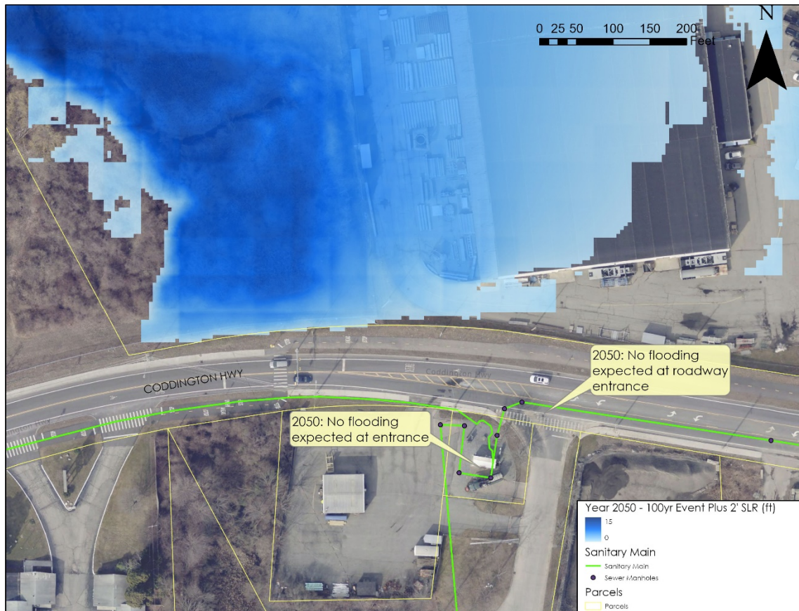
Figure 2. Projected water surface elevations around the Coddington Highway Pump Station for a 100-year coastal flooding event in the year 2050, factoring in 2 ft of sea level rise (SLR). Flood projections calculated by Coastal Resources Management Council (CRMC) STORMTOOLS, presented as water depth in feet above grade.
