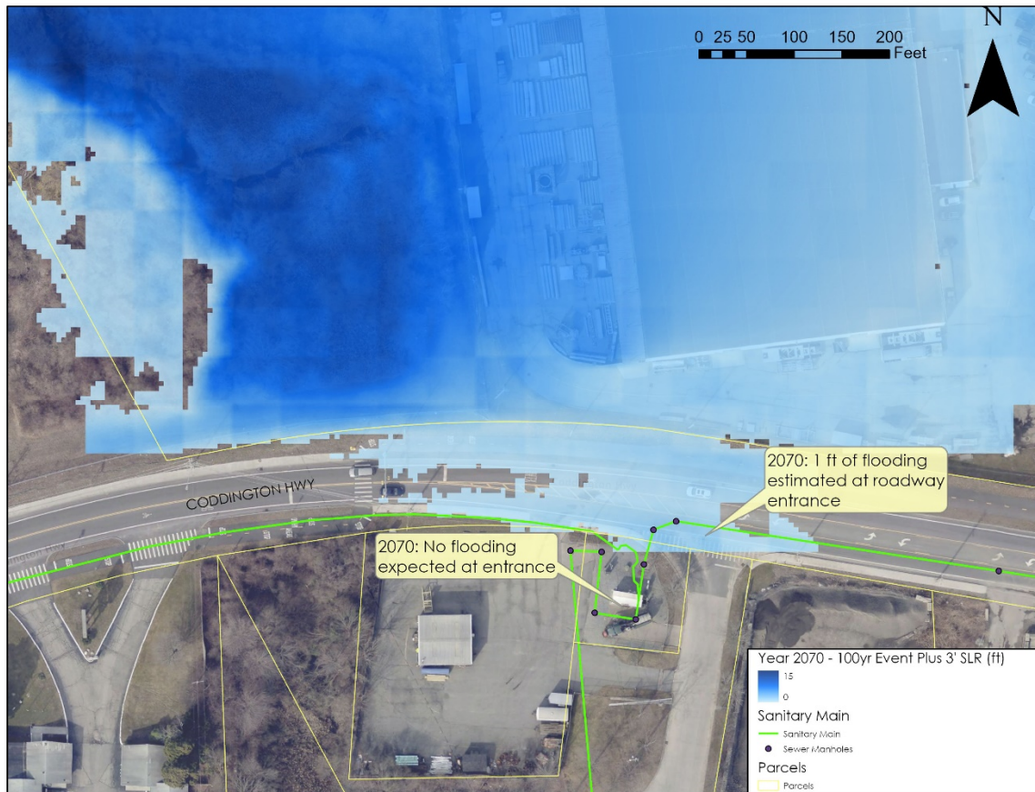
Figure 3. Projected water surface elevations around the Coddington Highway Pump Station for a 100-year coastal flooding event in the year 2070, factoring in 3 ft of sea level rise (SLR). Flood projections calculated by Coastal Resources Management Council (CRMC) STORMTOOLS, presented as water depth in feet above grade.
